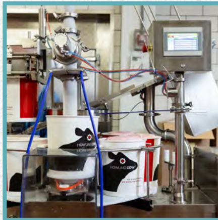
Tub indexes to filling station where it is filled, tub spins for even filling.
