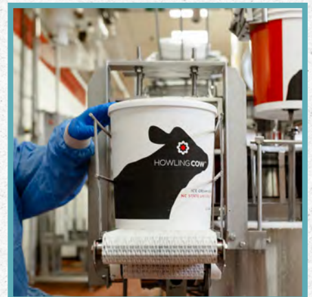
Finished 2.75 gallon tub exits filler on discharge conveyor ready for the freezer.
