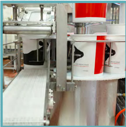
Tub dispenser de-nests a stack of cups.
