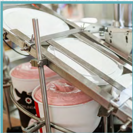
Lids are de-nested from stack and slide down chute for application.
