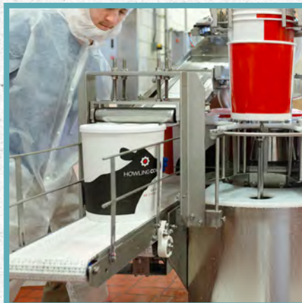
Lid is wiped onto tub and snaps over rim of tub.
