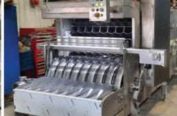
Stanpac is excited to partner with **Central Fabricating**, an industry leader in industrial equipment design and fabrication to offer a line of automatic bottle washers. There are currently 6 models available with speeds ranging from 30 to 80 bottles per minute.
